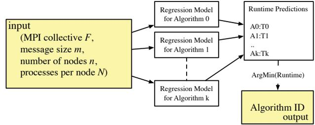
Fig. 3: General algorithm selection strategy for MPI collectives. The running time of each algorithm ( $1 \dots k$ ) is predicted for a given instance  $(F, m, n, N)$ . The algorithm with the smallest predicted runtime is selected.
