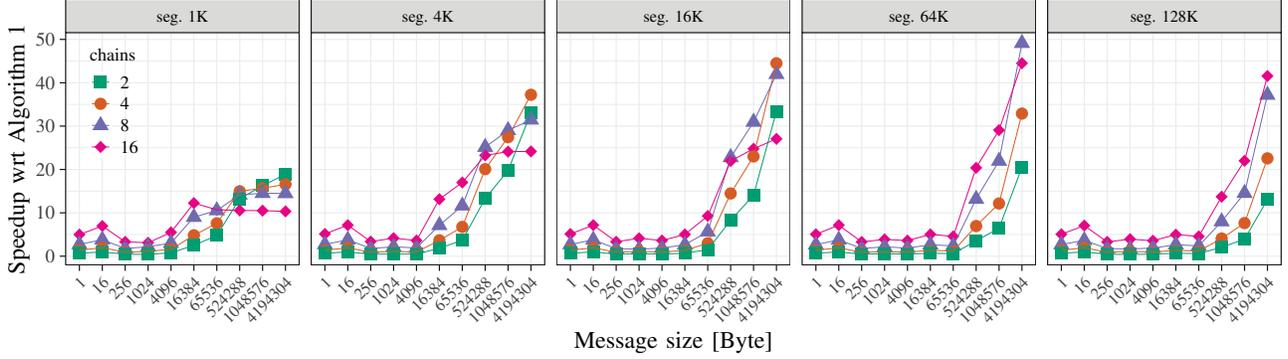
Fig. 2: Speed-up of various algorithmic configurations of alg. 2 (chain algorithm) with respect to alg. 1 (linear) of MPI\_Bcast; “seg.” denotes the segment size while “chains” denotes the number of chains;  $32 \times 32$  processes, Open MPI 4.0.2, Hydra.
