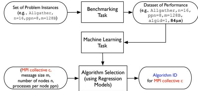
Fig. 1: Overall framework to solve the algorithm selection problem for MPI collectives.
