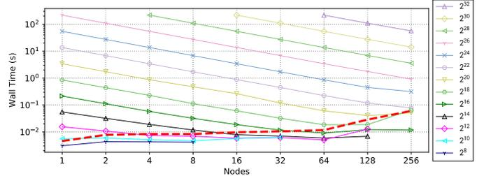
Figure 5: MPI strong scaling with problem size (stencil).
