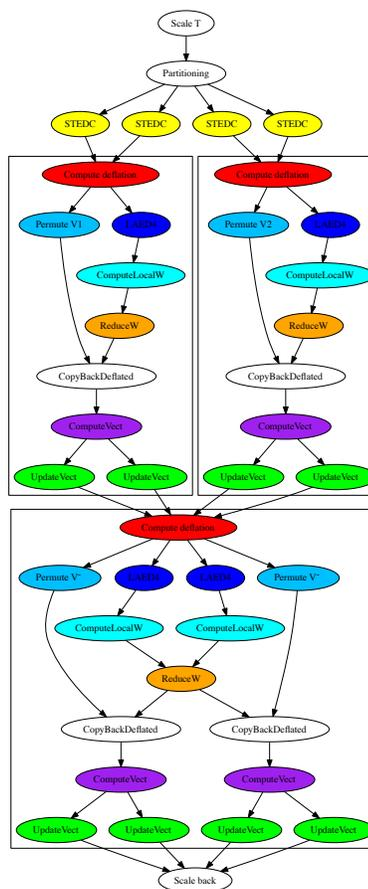
Figure 2. DAG of the D&C tridiagonal eigensolver for a matrix of size 1000, with a minimal partition size of 300, and a panel size of 500
