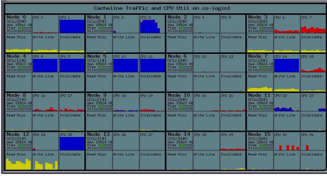
Figure 2: A screen shot of a performance monitoring tool on SGI Altix. The light yellow area reflects how many number of remote memory accesses have occurred.
