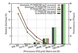
Cost of ABFT comes only from extra flops (to update checksums) and extra storage Cost decreases with machine scale (divided by Q when using  $P \times Q$  processes)
