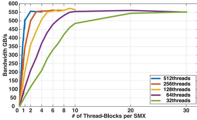
Fig. 1. The achievable bandwidth based on the number of TBs per SMX and the number of threads in each TB on the NVIDIA P100 GPU. Note: to obtain the total number of TBs running on the whole GPU, the  $x$  axis value should be multiplied by 56 since the P100 has 56 SMXs.
