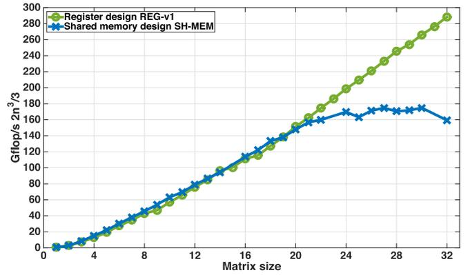
Fig. 7. Performance comparison of SH-MEM versus REG-v1 for the LU factorization on an NVIDIA P100.
