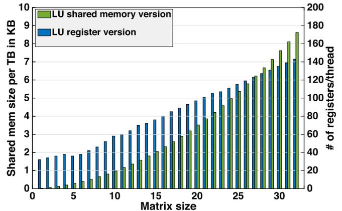
Fig. 4. The amount of shared memory (in KB) required by the SH-MEM design (left  $y$ -axis) and the amount of registers per thread required by the REG-v1 design (right  $y$ -axis) for the LU factorization in double precision for matrices ranging from  $2 \times 2$  to  $32 \times 32$  on an NVIDIA P100 GPU.
