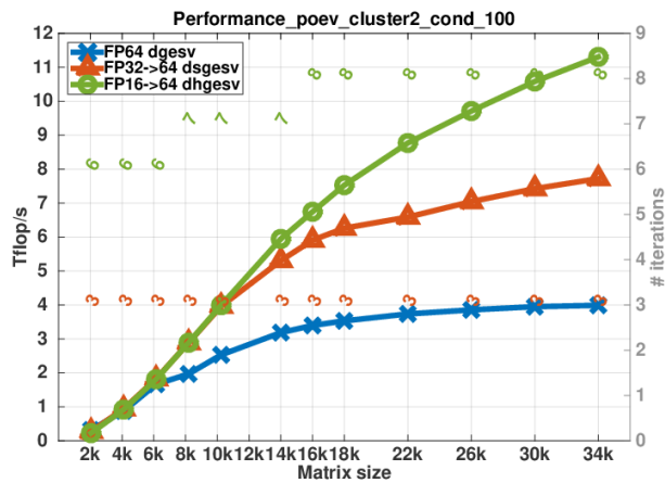
(c) matrix with positive \lambda and with clustered singular values, \sigma_i=(1, \dots, 1, \frac{1}{cond})
